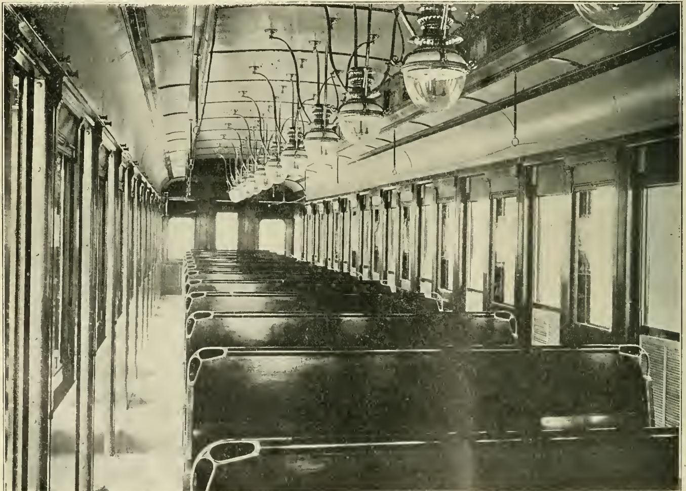
INTERIOR VIEW OF CAR TO SHOW CENTRAL ARRANGEMENT OF SEATS. NEW STEEL-FRAME, SIDE-DOOR SUBURBAN PASSENGER CARS.—ILLINOIS CENTRAL RAILROAD. DESIGNED BY A. W. SULLIVAN AND WILLIAM RENSHAW.
